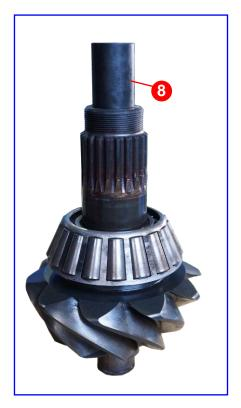
Step 1: Install No.8 on the shaft.
