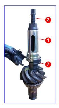
Step 3: Screw the No. 2 into No. 1, and hitch the bearing by No. 7.
