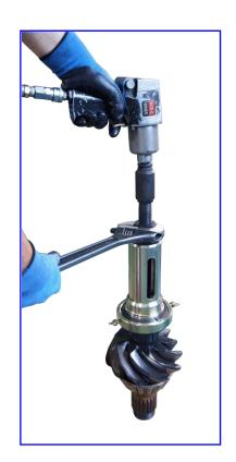
**Step 5:**Use the air impact tool to remove the bearing.
