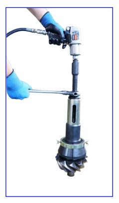
**Step 5:** Use the air tools, then you can remove the bearing.
