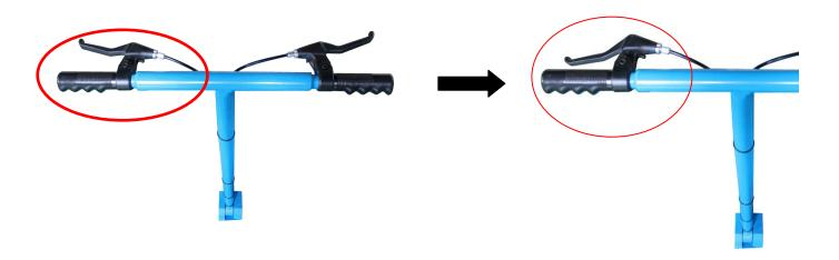
The left brake control safety device can be separated by pressing down. Please press it to the end to release. Under normal conditions, it is in close contact state (as shown below)
