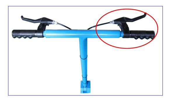
The right brake controls the angle of the rod. When the pressure is pressed, the machine can be adjusted at an appropriate angle (as shown below).
